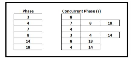
This ring structure allows for normal 8 phase operation, for individual northbound or southbound trains, and for northbound and southbound simultaneous trains.
