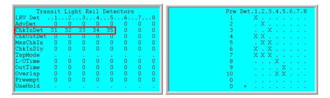
As an example, the user has programed the standard preemption hierarchy where HP1 overrides HP2, overrides HP3, etc. Below are screens for MM->5->9.>8, the Transit Check-in detectors, and MM->5->9->5 the Transit Preemption detector Matrix:
