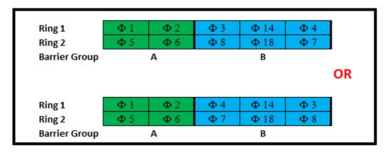
The "A" barrier group concurrencies remain unchanged and the sequences can have any combination of lead-lead, lead-lag, lag-lead, or lag-lag. The "B" barrier group concurrencies are:
