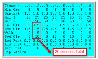
4) Scenario 4: **TLRD #3** using **PSD**. The Preemption Service Delay (**PSD**) Mode is intended for use with an input coming from external source like a rail cabinet or GPS. It is automatically calculated by the software. Please note that the **PSD** time is calculated using the phase which has to the longest programmed time:
