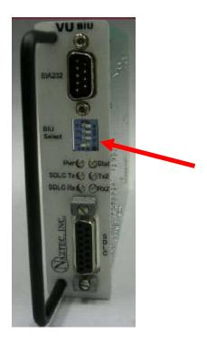
Please note that once the user chooses the BIU select switch selected, the detector numbers that will automatically be chosen that correspond to that BIU (see section 1b above). This selection must also be used as zones\output numbers on the VU1F / VU2F configuration when you create your detection zones.
