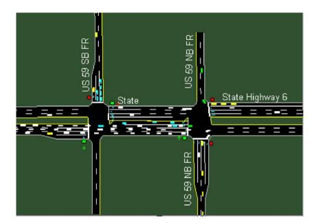
In this example, our offset is referenced to the beginning of phase 2 which is the WBT (westbound through movement) entering the interchange from the east traveling west. The phasing orientation is based on how the controller is actually phased on the street - Synchro can model whatever is there. Also notice that the interchange is the "Master Intersection" for the network. This setting insures that the offset is synced to 0.0" and the rest of the network is referenced to this intersection.
