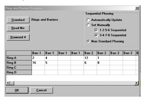
The "Diamond 4" button in the *Ring and Barrier Designer* was used to select the phase sequence shown above for a 4-phase diamond intersection. Search on the "diamond" in Synchro's help file to read more about Group Control. Sympholic phasing schemes for a diamond interphance are based on
