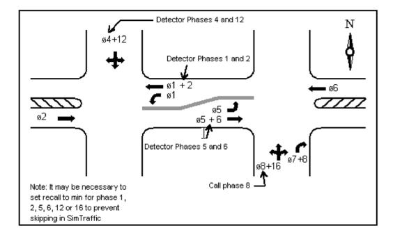
Work through "SETTING UP A TIMING PLAN" in Synchro's help file which is a step-by-step tutorial on how to set up *Group Control* and phase the intersections for your interchange model. If you don't set the controller type as "Pretimed", you will need to be sure to code the detectors necessary to drive all of the phases in your model, or else you will create a lot of "slack time" from the actuated phases when you view your model in SimTraffic.
