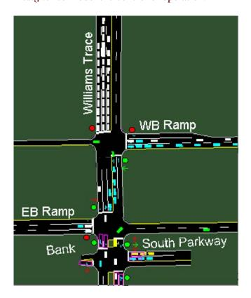
Synchro is used to adjust the split times for the WB and EB Ramps (with "Lock Timings" turned off). Then the timings are locked as shown below and Synchro is used to adjust the offsets with the rest of the network (30 intersections in this case).
