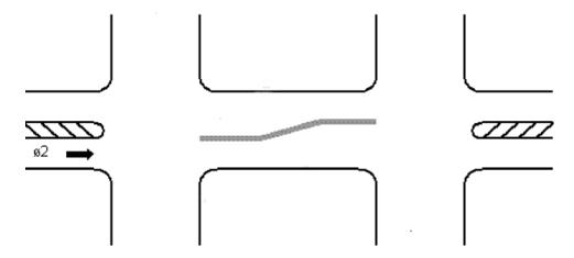
Now, does the *Ring and Barrier Designer* above make more sense? Can you follow the sequence from 2+16 to 4 to 6+12 to 8? Again, the interior phases 1 and 5 are just "helper phases" to insure that the through movement downstream is progressed through the interchange.
