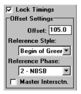
The additional coding needed to correctly model the frontage road signals in Synchro is provided below. You must "Lock" these Group Control intersection as part of a larger network.
