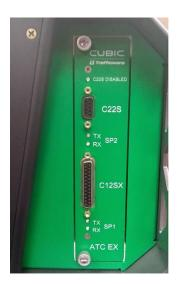
ATC Cabinet Card must be plugged in before COMMANDER is powered up.
