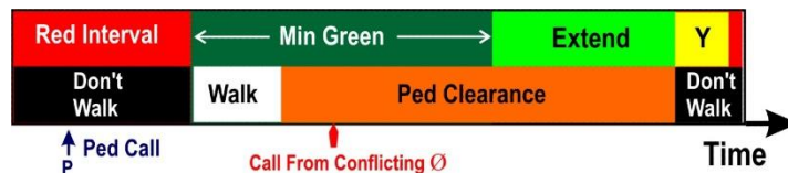
Ped Clearances Ends Prior to Vehicle Clearance if PedClr-Thru-Yellow is Not Enabled
