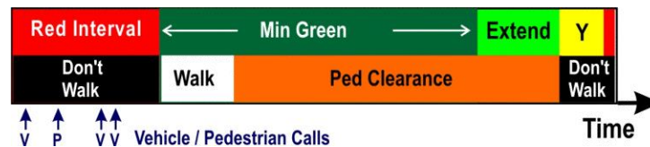
Vehicle and Pedestrian Detectors Place a Service Demand on the Phase
